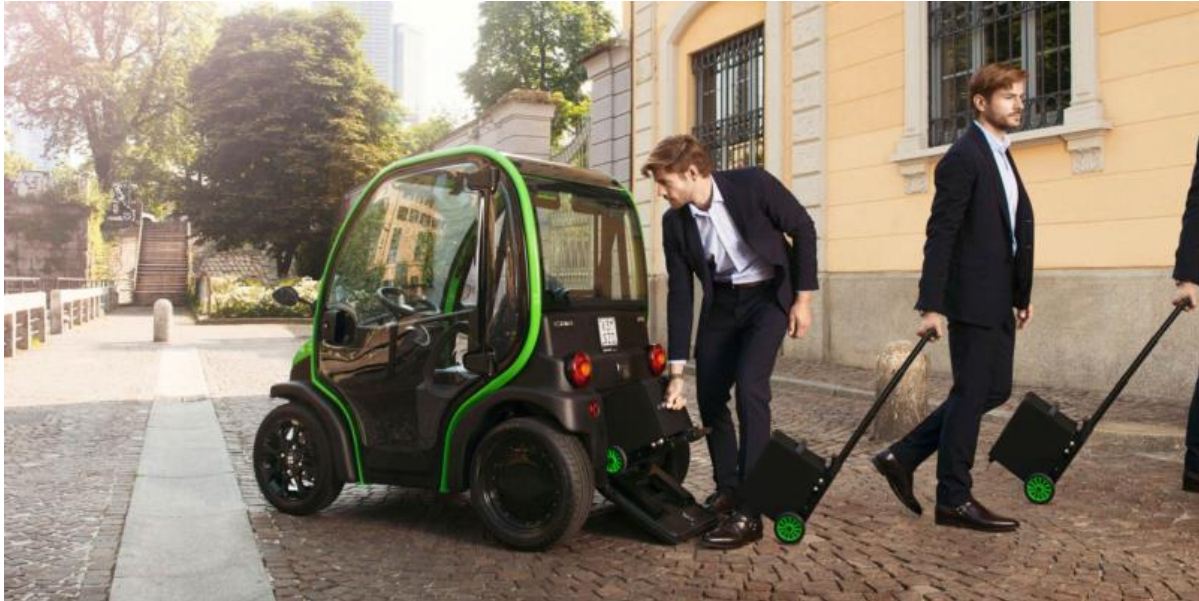
Figure 0.36. Examples of electric quadricycles with removable battery
